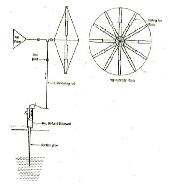
Figure no. 1. High solidity wind turbine with No. 6 hand tube well
