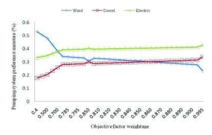
Figure no. 6. Pumping system preference measure with respect to objective factors weight-age
